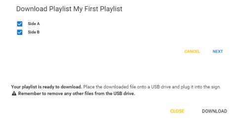
Find the downloaded file, which will end with .package, and copy it onto an empty USB drive. Take the USB drive out to your sign and plug it into the external USB port, if equipped. A confirmation message will briefly appear on the sign's display. Wait until the message says to remove the device, and take the drive out of the port. Your sign should now be updated with the new playlist.
